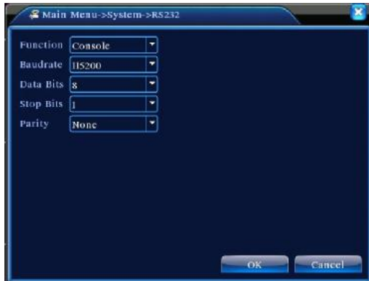
Pic 4.39 serial port setting
