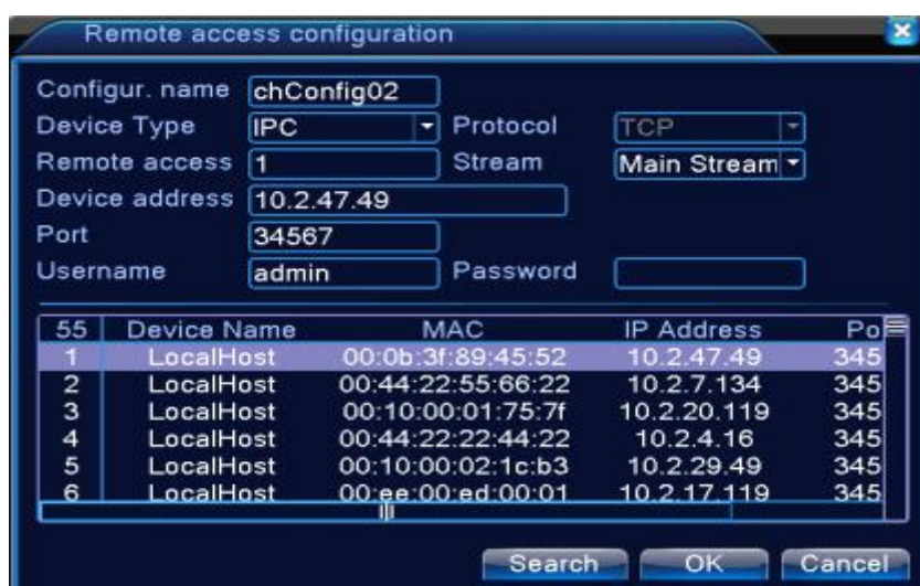
Pic 4.45 the device list searched under remote channel setting
