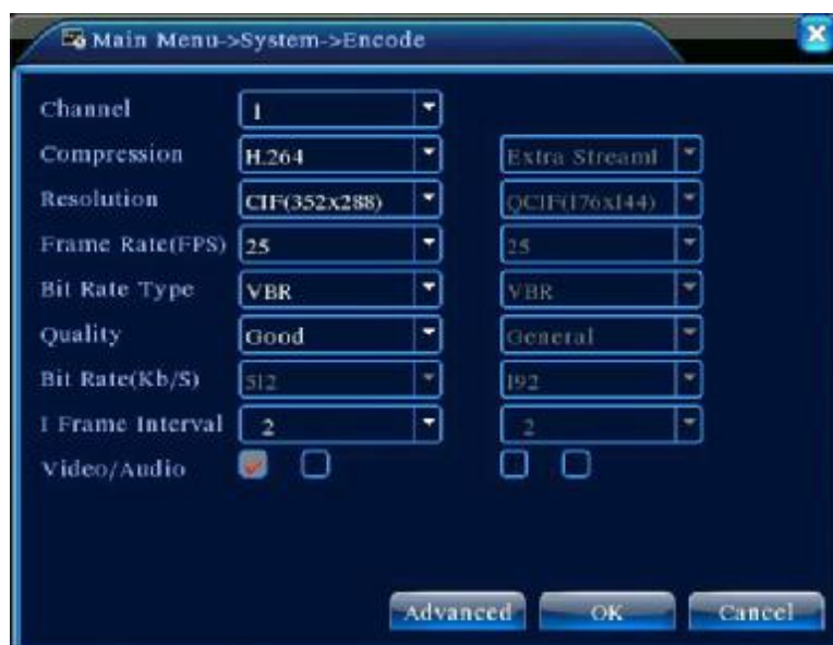
Picture 4.20 Encode setup
